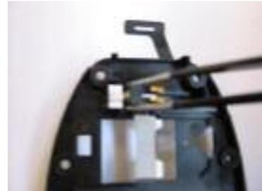
Remove the PCB with antenna assy
