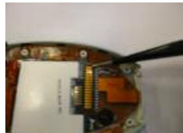
Remove the LCD assy with tweezers
