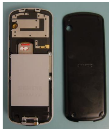
Remove Battery cover.
