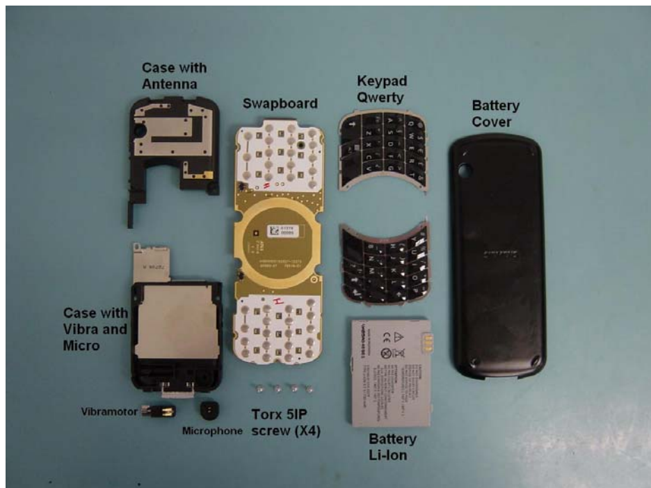
Fully disassembled SK65 (Lower parts)
