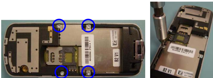
Remove the 4 screws (as indicated) with T5 Plus screw driver (set Torque = 16 cNm).
