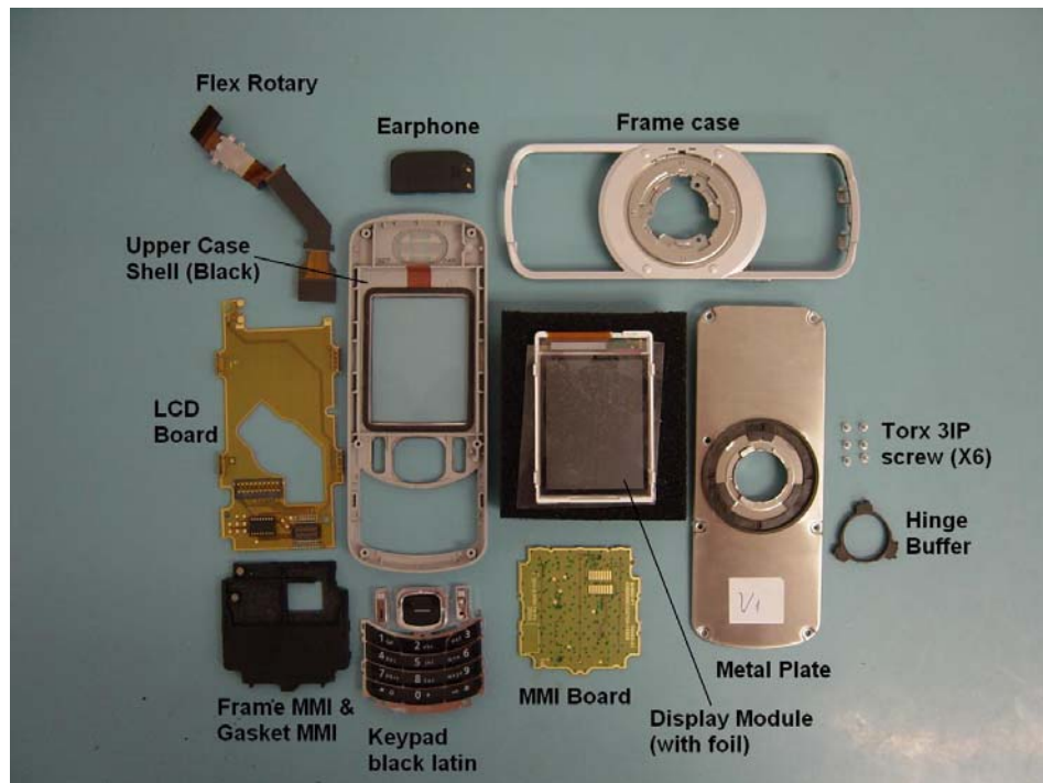
Fully disassembled SK65 (Upper parts)
