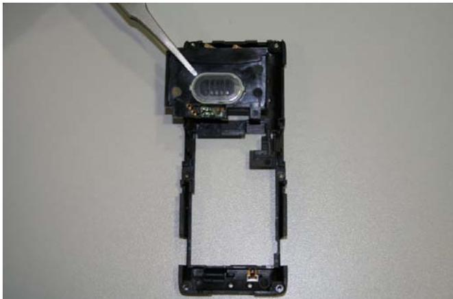
Assemble Ringer by using Tweezers.
