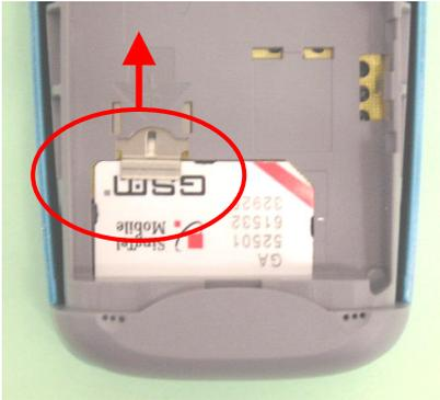
To remove the SIM card, push the SIM slider upwards as indicated by the arrow.
