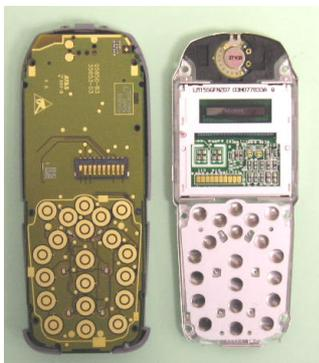
The RF board (PCB) can be seen after removing the SAR Frame and Light Guide assembly.
