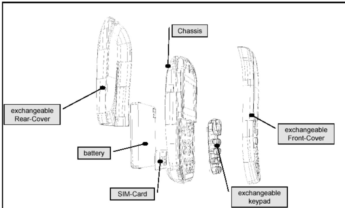
The C60 enables the customer to freely customize the outlook of their phone via the means of exchangeable Front/Rear covers as well as keypad.
