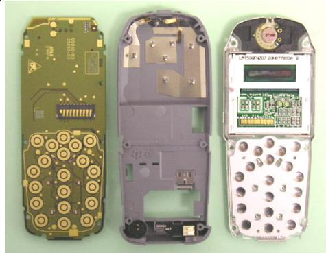
Separate the PCB from the Lower Mounting Frame. The antenna is built-in on the Lower Mounting Frame.
