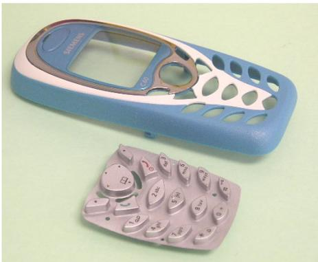
The keypad can be separated from the CLIPit cover.
