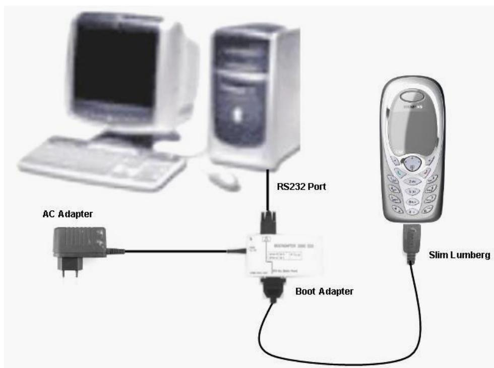
Figure 1. C60 Software Programming Setup
