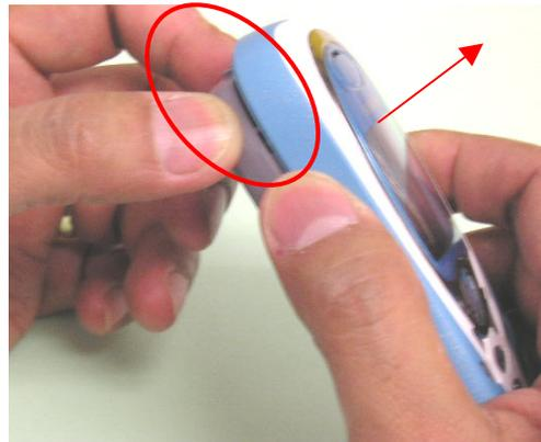
To remove the CLIPit cover, gently pull the cover upwards from the side of the phone while holding firmly the lower mounting frame as shown.
