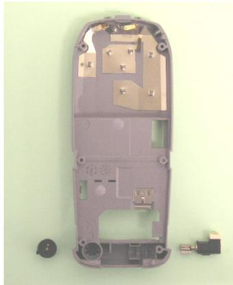
Remove the Vibrator motor and MIC from the Lower Mounting Frame.
