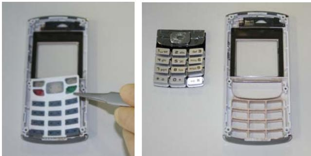
Remove keypad by using tweezers.
