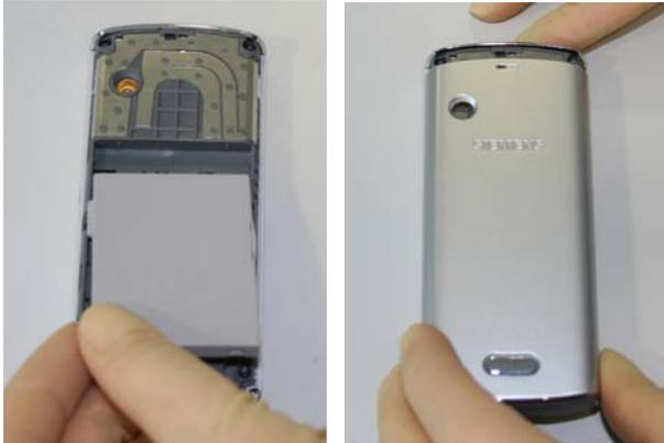
Assemble Battery and Battery Cover Assy.
