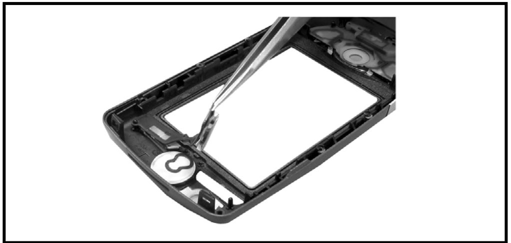
Figure 11. Removing and Replacing the Gaming Buttons
